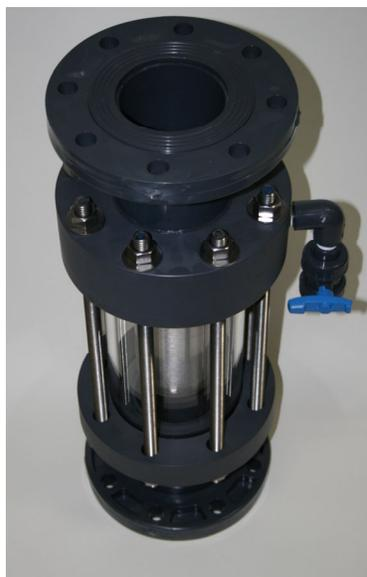
A resin trap is a very simple filtering device using a stainless steel wedge-wire filter. The slots are small enough to retain any upstream ion exchange resins or other filtration media. At the same time, the number and size of the openings must be sufficient to keep the pressure drop to a minimum. A clear sleeve will visually indicate whether there is an upstream problem. A small ball valve allows for removal of resin or media after the problem has been repaired.
