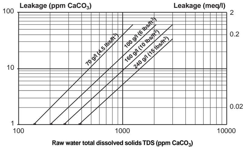
Figure 2. Operating Capacity of DOWEX HCR Resin for Water Softening
