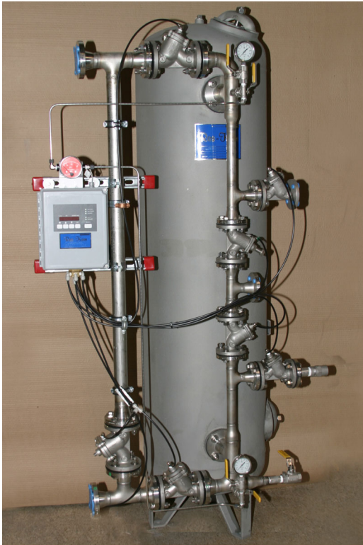
Figure 1 Initial Design of Condensate Polisher
